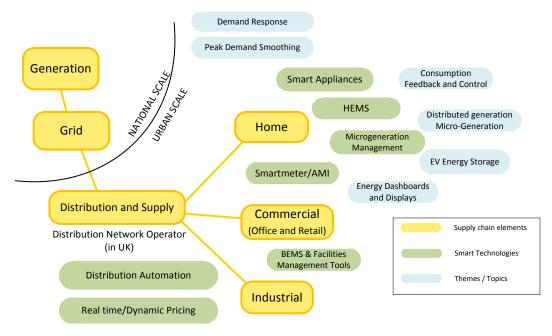
Figure 1.2: A generic energy market diagram, showing the elements of the supply chain (yellow) and the associated smart technologies (green). Wider smart energy management concepts are shown in blue. Source: Arup Analysis
