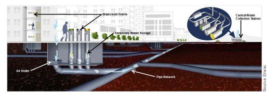
Figure 4.5: An illustration of an Automated Waste Collection Systems system Source: Envac
